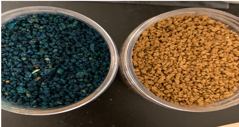
Figure 2. Coated and uncoated granules manufactured from brewers grains.
